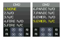
For example, if connecting with fire sensor, it should set 4. FIRE N/O or 5. FIRE N/C and it may cause fire alarm and icon in case of fire. In case of fire, the door automatically opens for safety.
