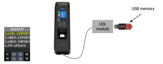
If Terminal detect UDL Device and USB memory, icon is displayed in the default screen.
