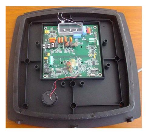
Here we can already see the back plastic case, of the AY-Z12, placed into the back case of the AY-Z12 Reader, and connected to the Antenna Litz Wire. You cannot see the Antenna, because it is covered by potting material.
