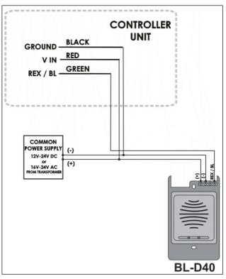
Figure 4: Wiring Diagram for the BL-D40 External Sounder
