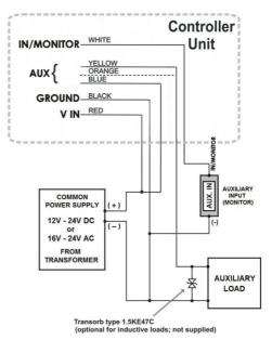
Figure 3: Wiring Diagram for Auxiliary Input & Output
