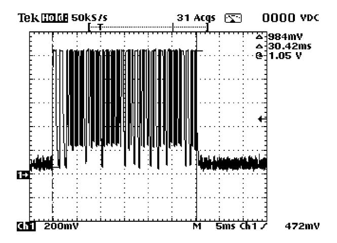
Pulse train duration = 30.42 msTx on =  $30.42 \times 0.5 = 15.21 \text{ ms}$ Average factor =  $20 \log 15.21/100 = -16.35 \text{ dB}$
