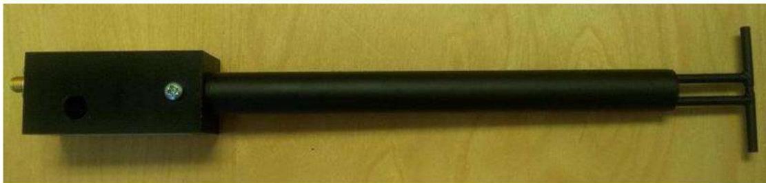
Figure 1 – MVG COMOSAR Validation Dipole
