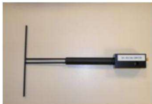
Figure 1 – Satimo COMOSAR Validation Dipole
