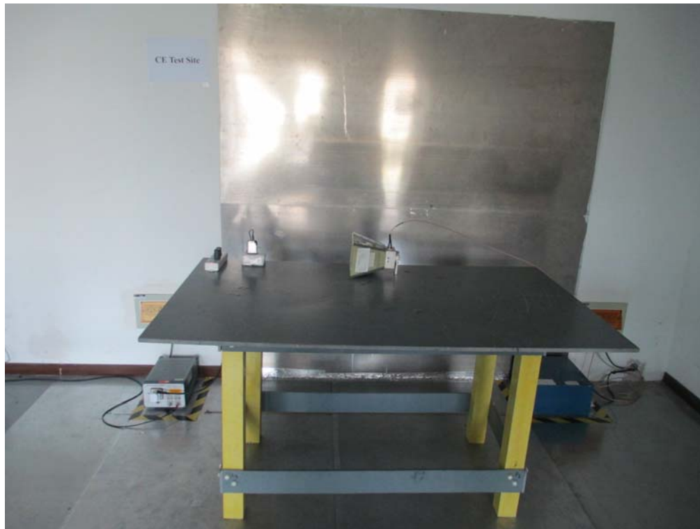
Conducted Emissions Test Setup Front View
