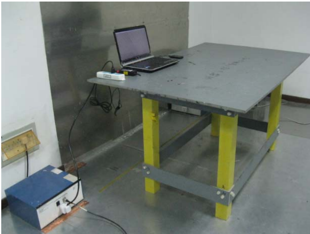
Conducted Emissions Test Setup - Side View
