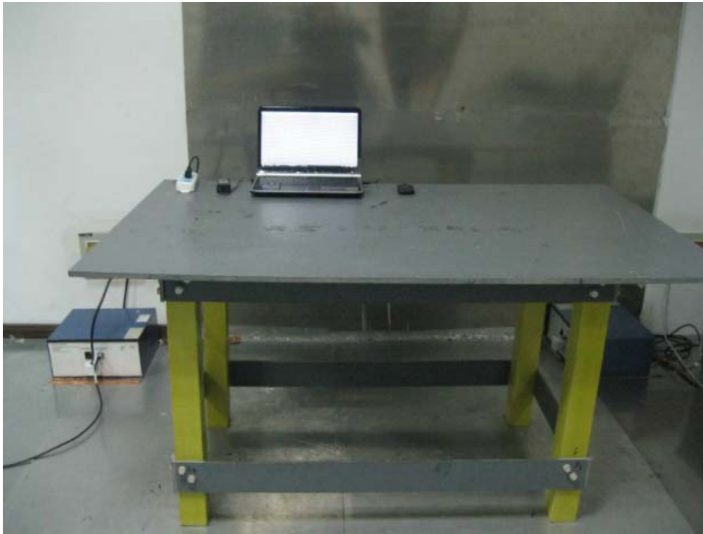
Conducted Emissions Test Setup - Front View
