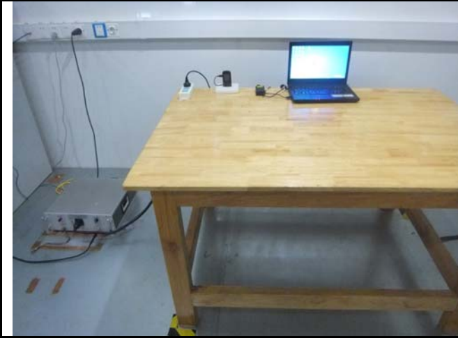
Conducted Emissions Test Setup – Front View
