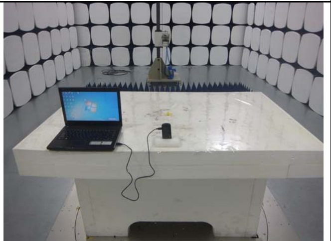
Radiated Spurious Emissions Test Setup Above 1GHz
