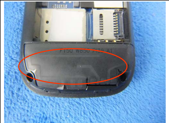
GSM/PCS/UMTS-FDD Antenna View
