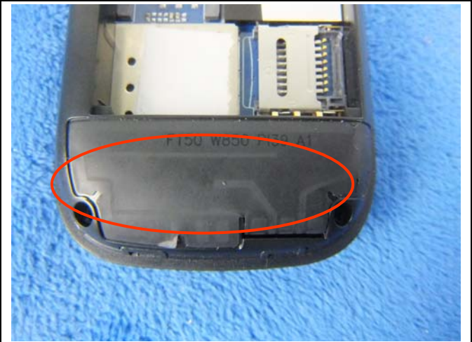
GSM/PCS/UMTS-FDD Antenna View
