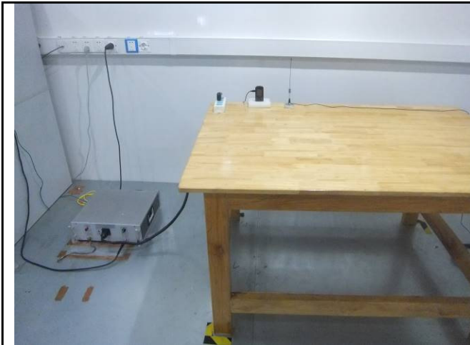
Conducted Emissions Test Setup Front View
