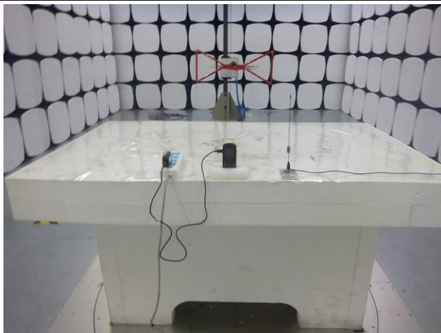
Conducted Emissions Test Setup Front View
