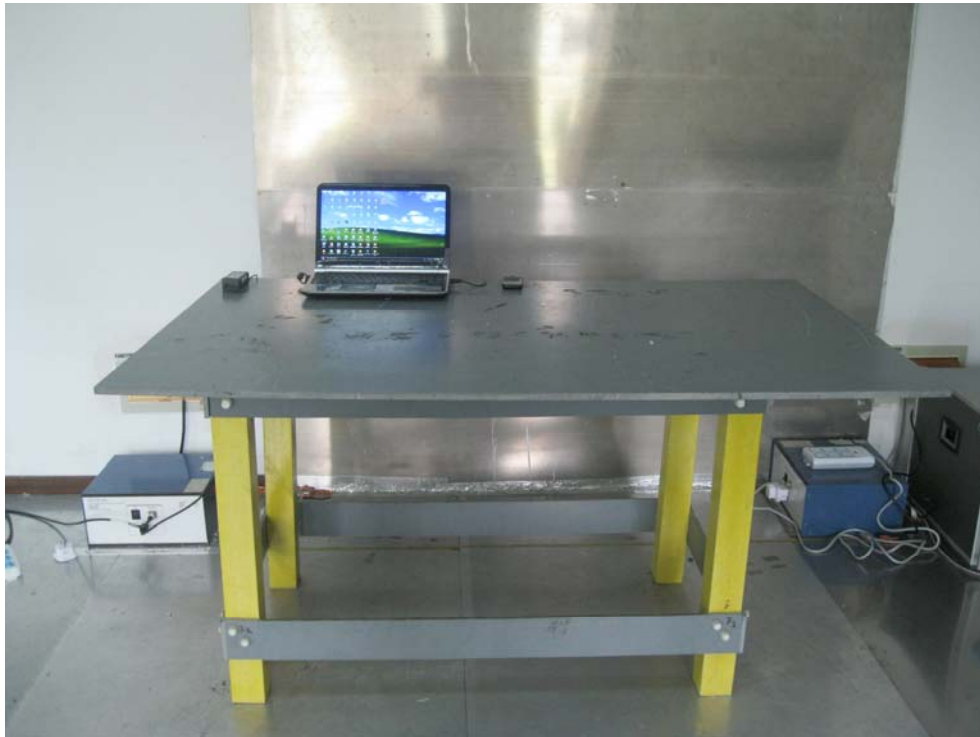
Conducted Emissions Test Setup - Front View
