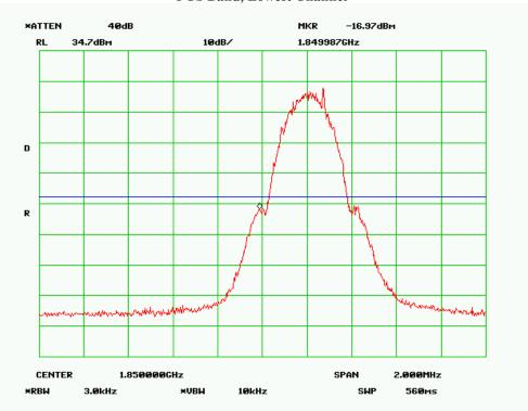
Note: offset= cable loss + 10log(1%\*26dB/3kHz) offset=  $4.7+10\log(3.17/3) = 4.94dB$
