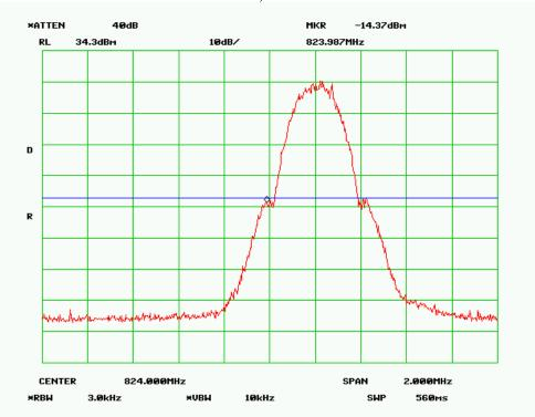
Note: offset= cable loss + 10log(1%\*26dB/3kHz) offset=  $4.3+10\log(3.18/3) = 4.55dB$
