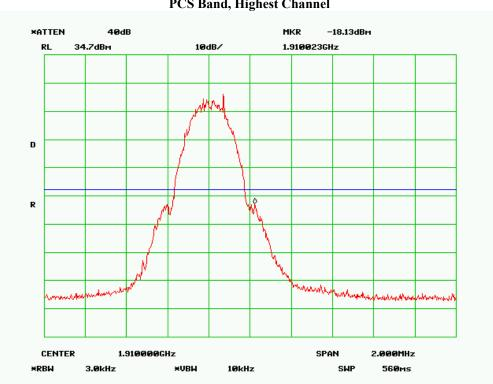
Note: offset= cable loss + 10log(1%\*26dB/3kHz) offset=  $4.7+10\log(3.13/3) = 4.88dB$
