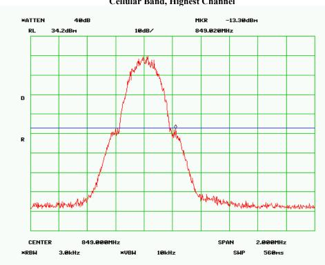
Note: offset= cable loss + 10log(1%\*26dB/3kHz) offset=  $4.2+10\log(3.17/3) = 4.44dB$
