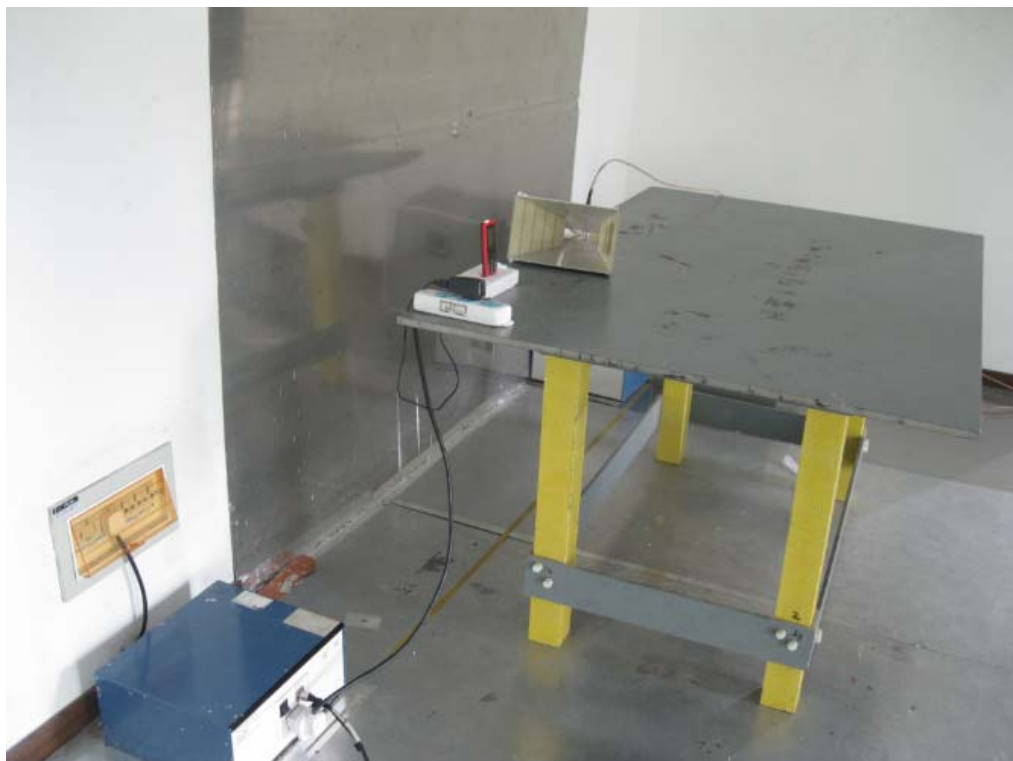
Conducted Emissions Test Setup - Side View
