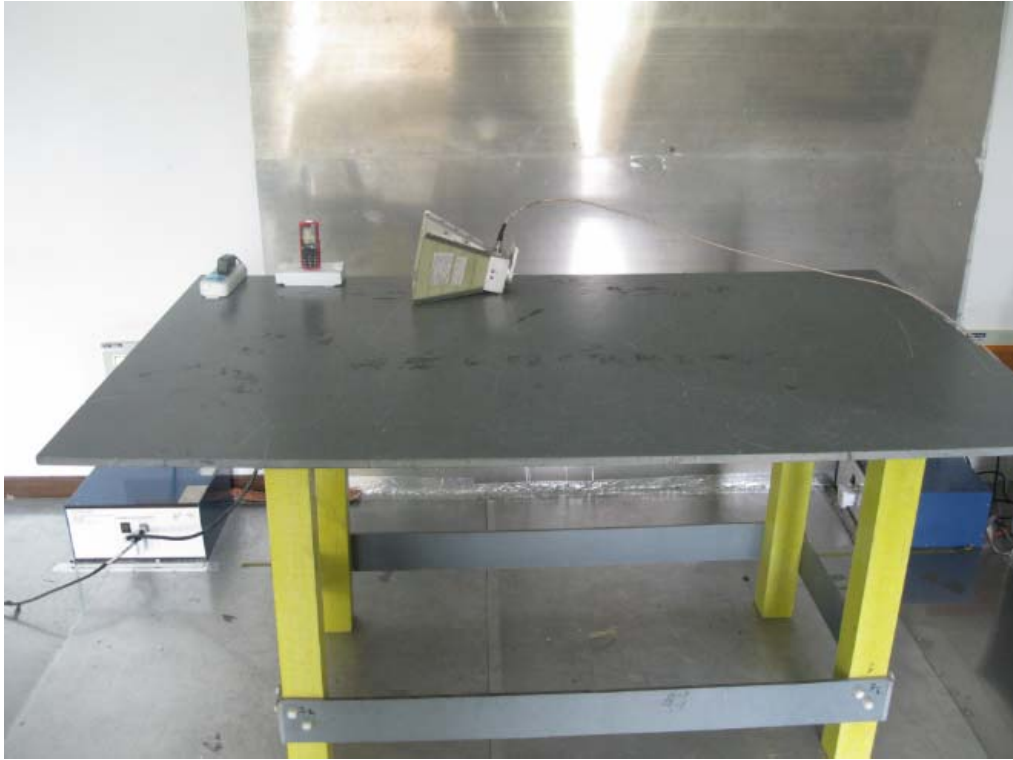
Conducted Emissions Test Setup - Front View
