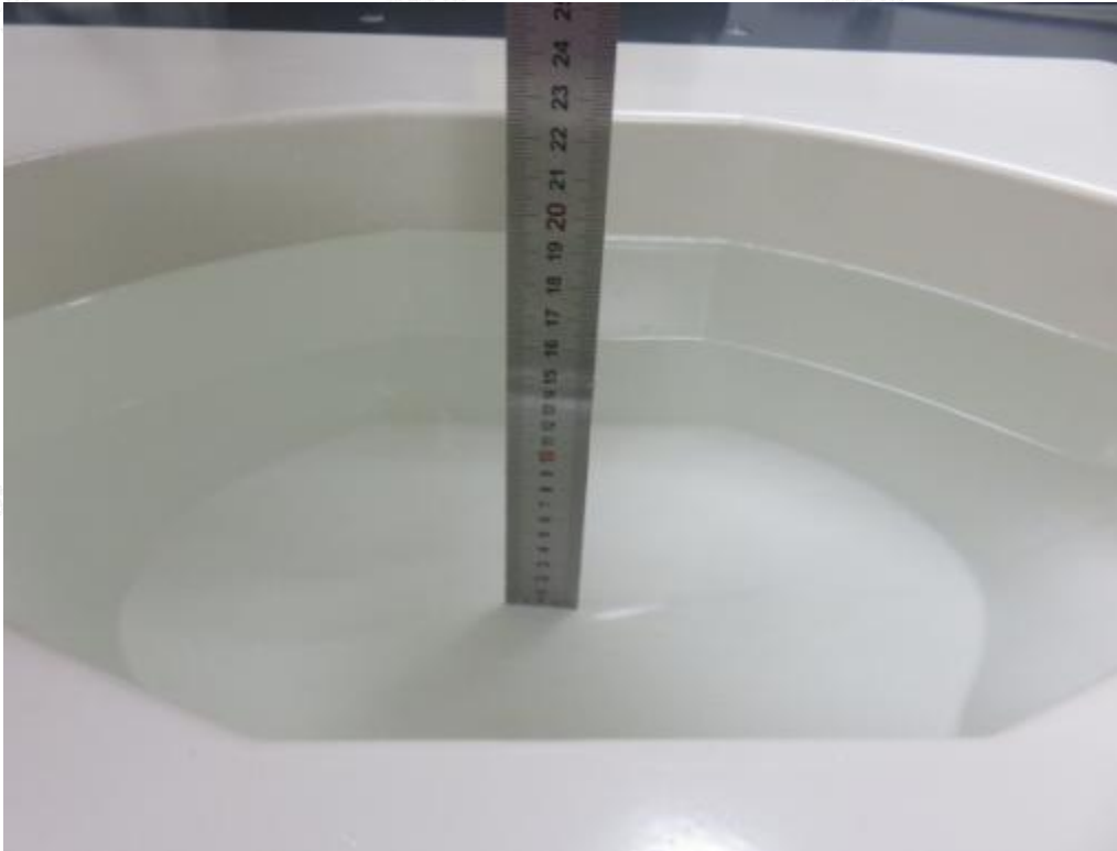
Photograph of the depth in the Body Phantom (1800MHz, 16.1cm depth)
