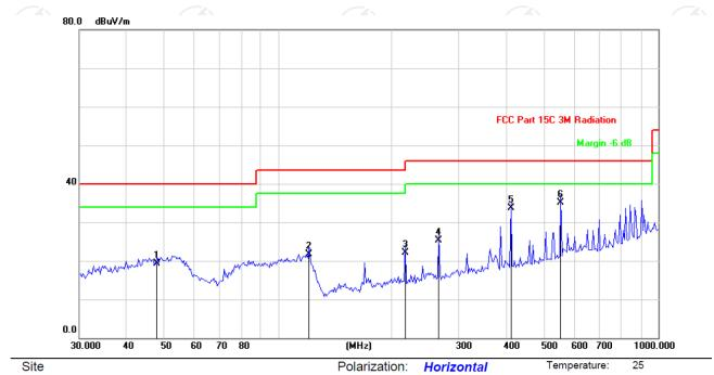
Limit: FCC Part 15C 3M Radiation Power: AC 120V/60Hz Humidity: 55 %
