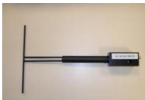
Figure 1 – Satimo COMOSAR Validation Dipole
