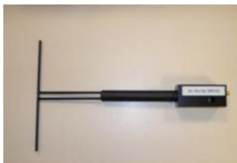
Figure 1 – Satimo COMOSAR Validation Dipole
