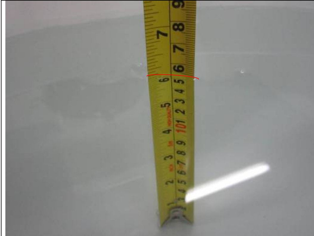
Liquid depth \geq 15cm
