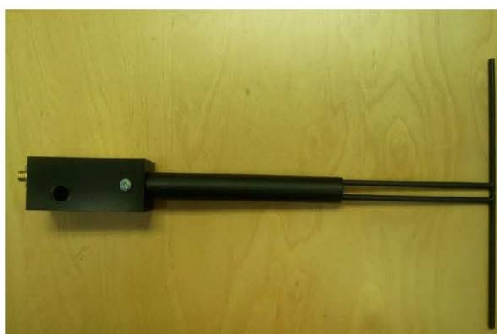
Figure 1 – MVG COMOSAR Validation Dipole
