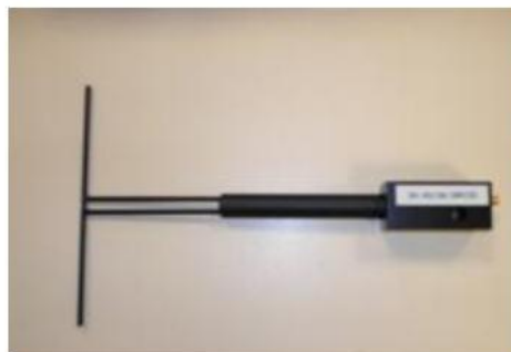
Figure 1 – Satimo COMOSAR Validation Dipole
