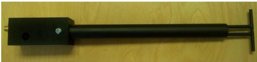
Figure 1 – MVG COMOSAR Validation Dipole
