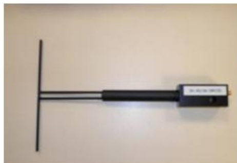
Figure 1 – Satimo COMOSAR Validation Dipole
