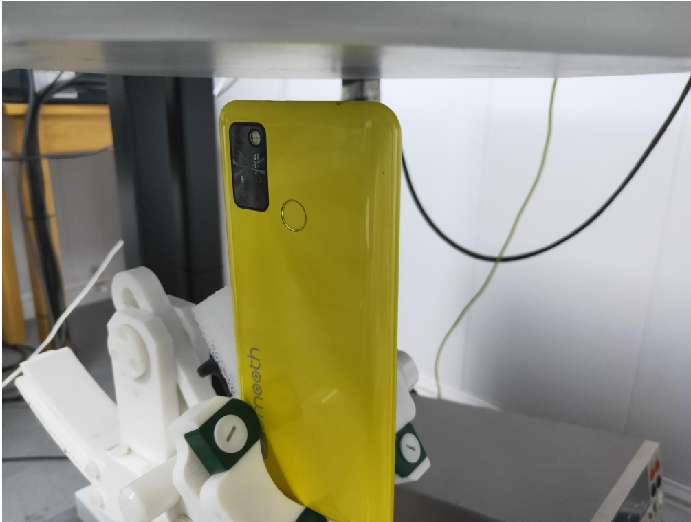
10mm body-worn Top Side Setup Photo (hotspot)
