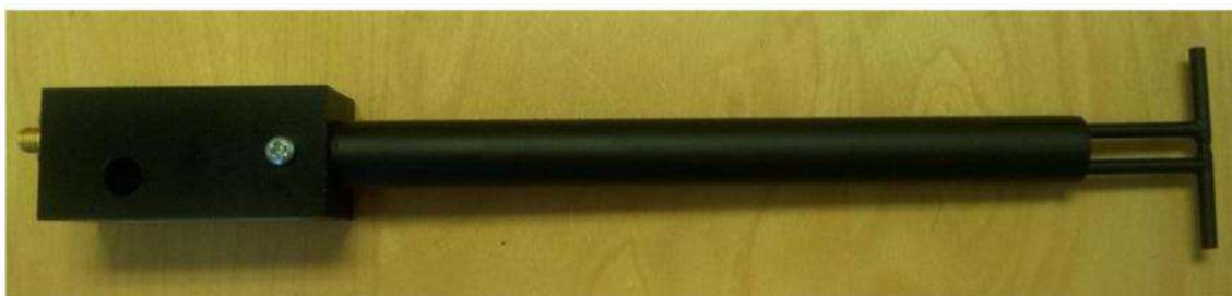
Figure 1 – MVG COMOSAR Validation Dipole
