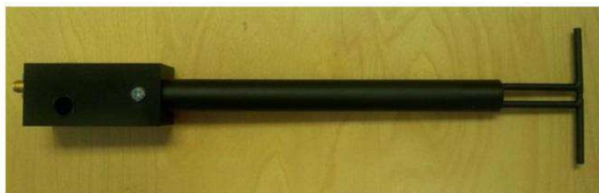
Figure 1 – MVG COMOSAR Validation Dipole
