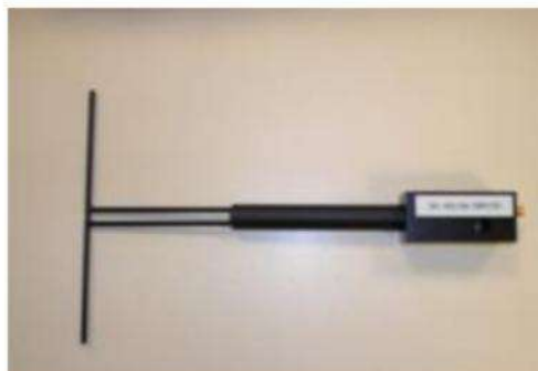
Figure 1 – Satimo COMOSAR Validation Dipole
