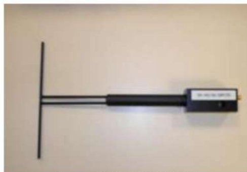
Figure 1 – Satimo COMOSAR Validation Dipole
