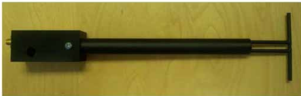
Figure 1 – MVG COMOSAR Validation Dipole
