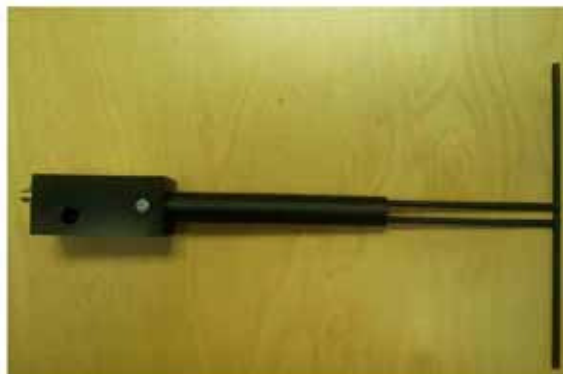
Figure 1 – MVG COMOSAR Validation Dipole
