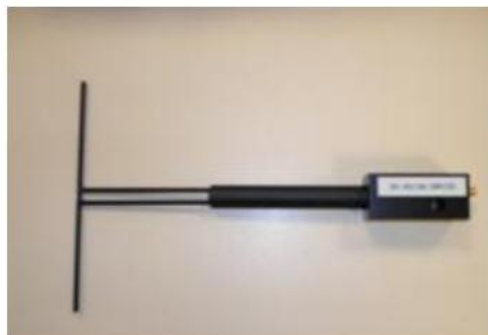
Figure 1 – Satimo COMOSAR Validation Dipole
