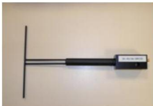
Figure 1 – Satimo COMOSAR Validation Dipole
