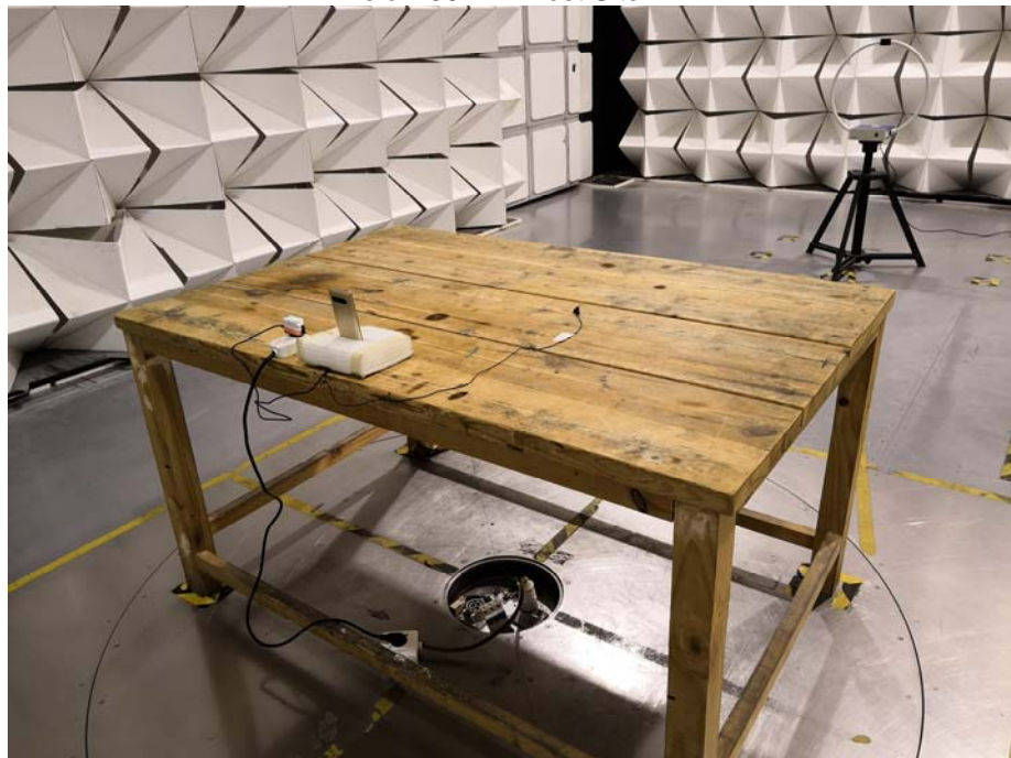
Below 30MHz Test Site 2#
