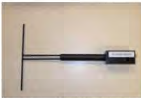
Figure 1 – Satimo COMOSAR Validation Dipole
