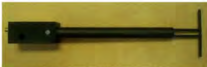
Figure 1 – MVG COMOSAR Validation Dipole
