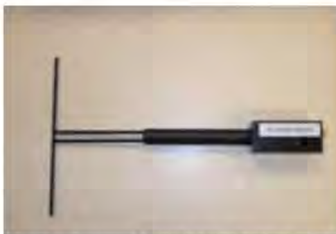
Figure 1 – Satimo COMOSAR Validation Dipole
