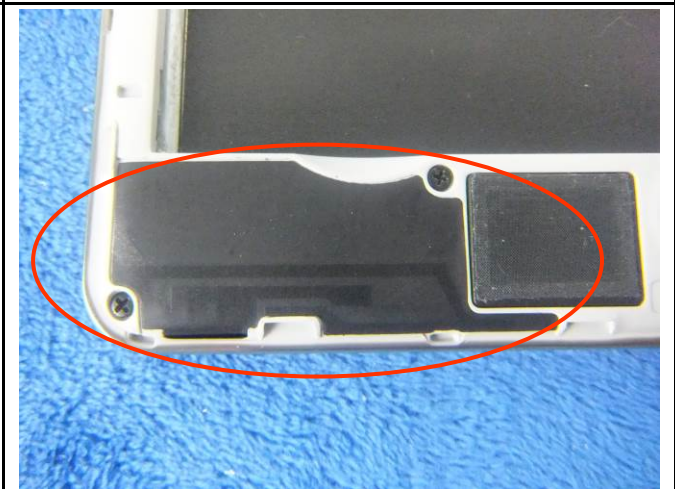
GSM/PCS/UMTS-FDD Antenna View
