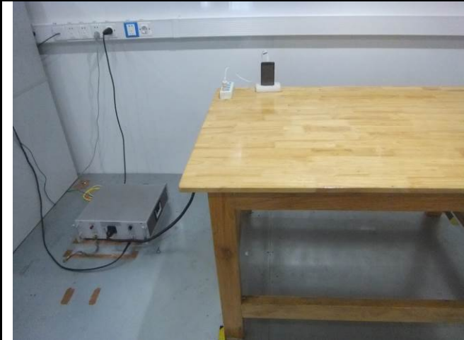
Conducted Emissions Test Setup Front View
