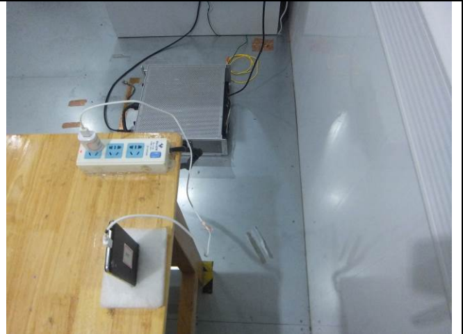
Conducted Emissions Test Setup Side View
