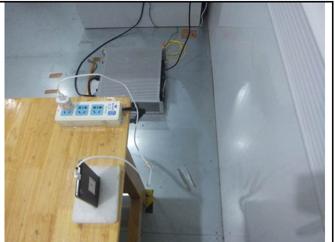
Conducted Emissions Test Setup Side View
