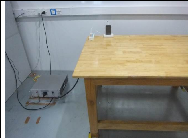
Conducted Emissions Test Setup Front View
