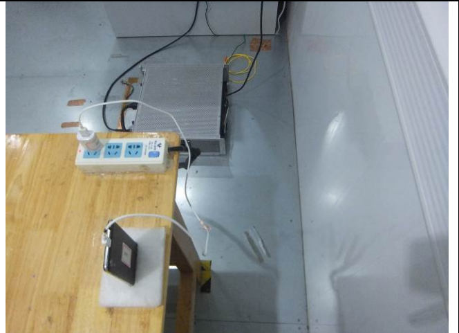
Conducted Emissions Test Setup Side View
