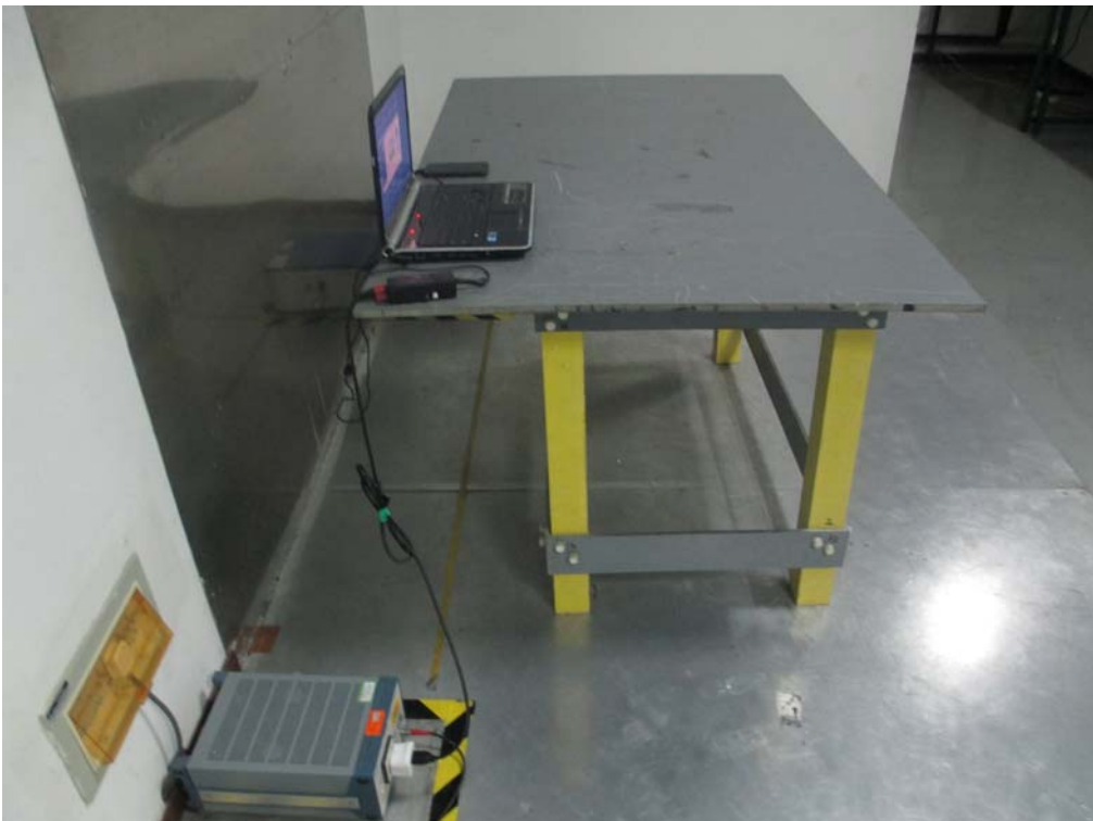
Conducted Emissions Test Setup Side View
