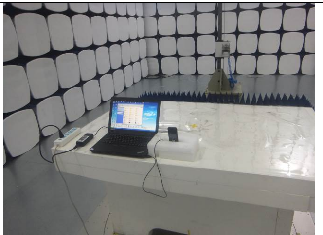
Radiated Spurious Emissions Test Setup Above 1GHz
