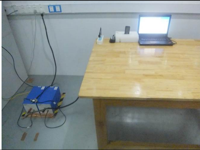
Conducted Emissions Test Setup – Front View
