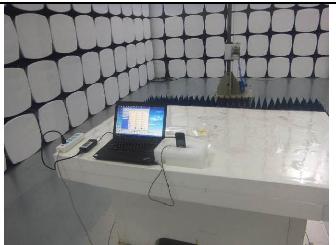
Radiated Spurious Emissions Test Setup Above 1GHz
