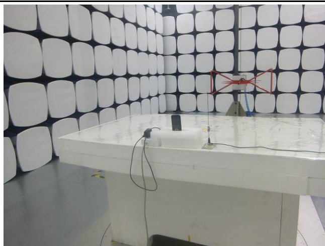
Conducted Emissions Test Setup Front View
