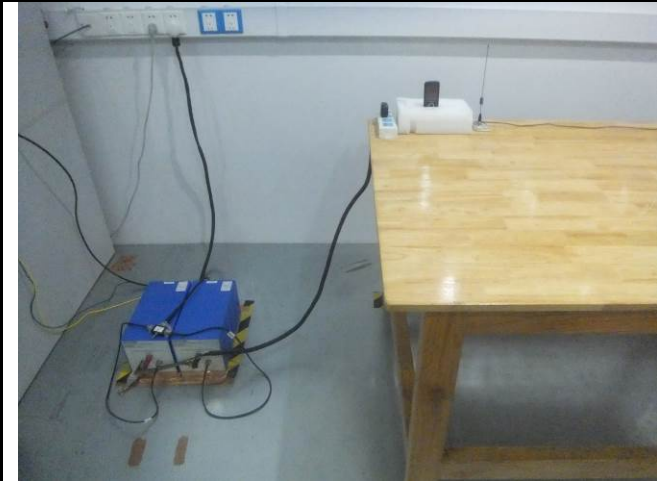
Conducted Emissions Test Setup Front View
