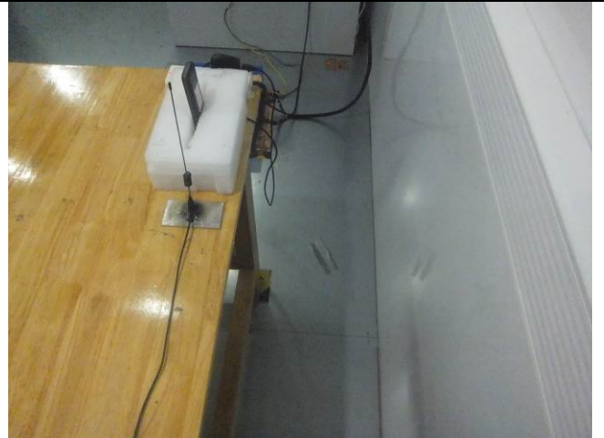
Conducted Emissions Test Setup Side View
