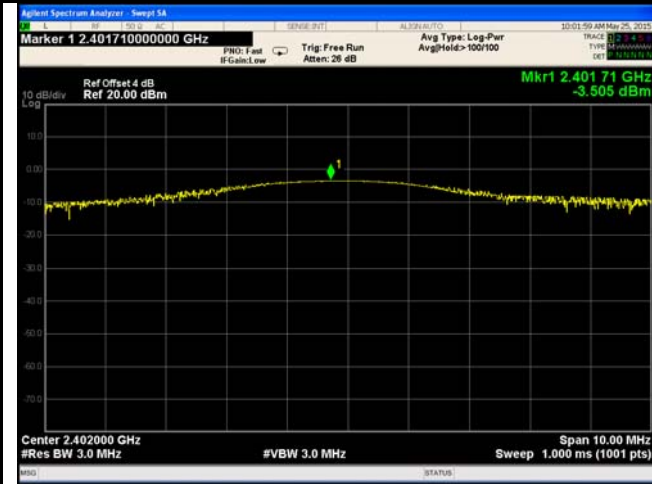
8DPSK Output power - Low CH 2402
