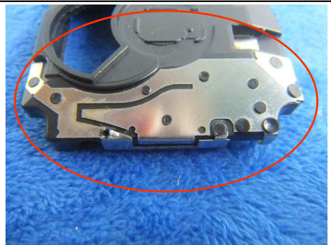
GSM/PCS Antenna View
