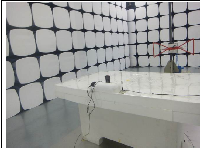
Radiated Spurious Emissions Test Setup Below 1GHz
