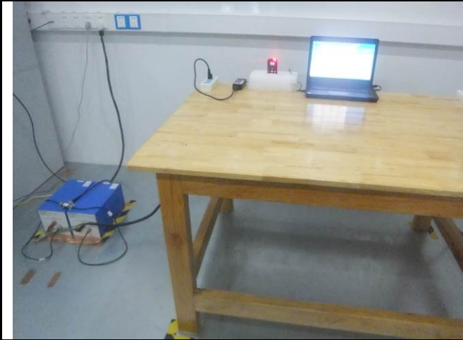
Conducted Emissions Test Setup – Front View
