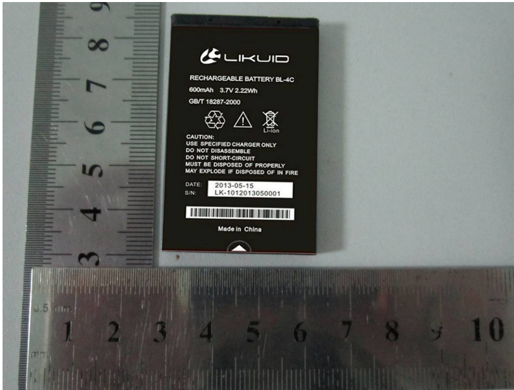
Battery- Front View
