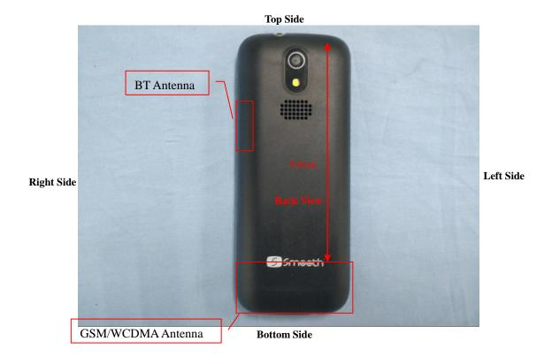
**Block Diagram for EUT Antenna Position**
