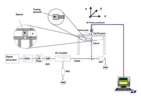
**System Verification Setup Block Diagram**
