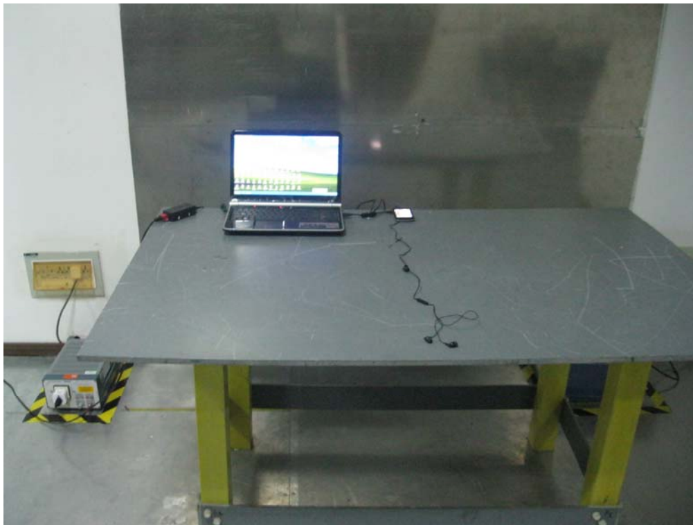
Conducted Emissions Test Setup Front View
