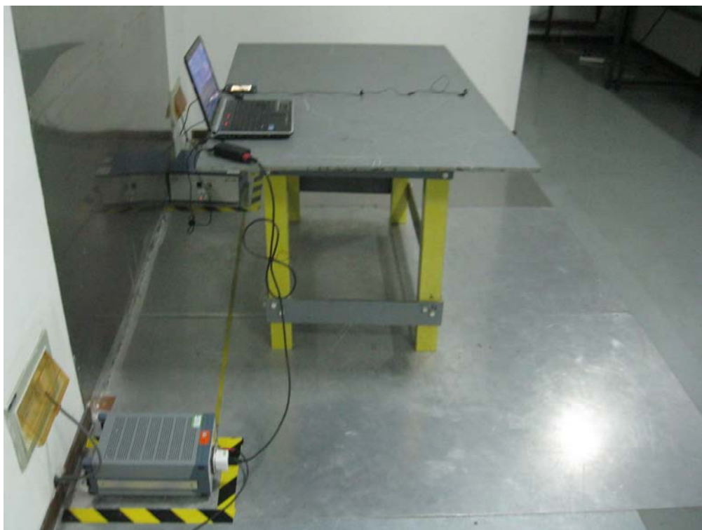
Conducted Emissions Test Setup Side View
