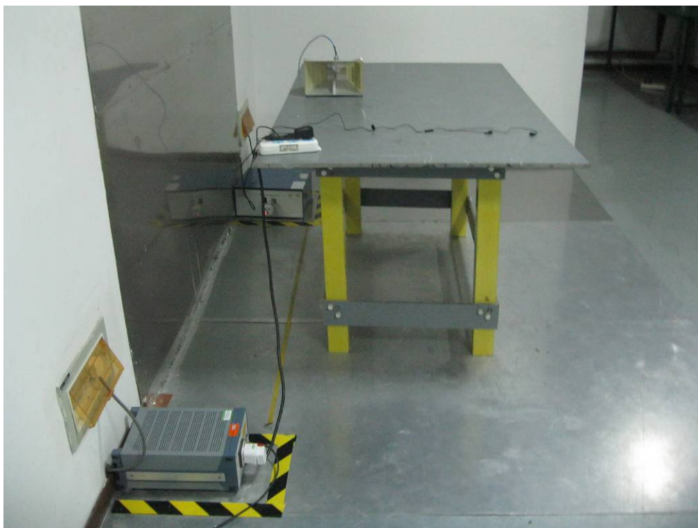
Conducted Emissions Test Setup Side View
