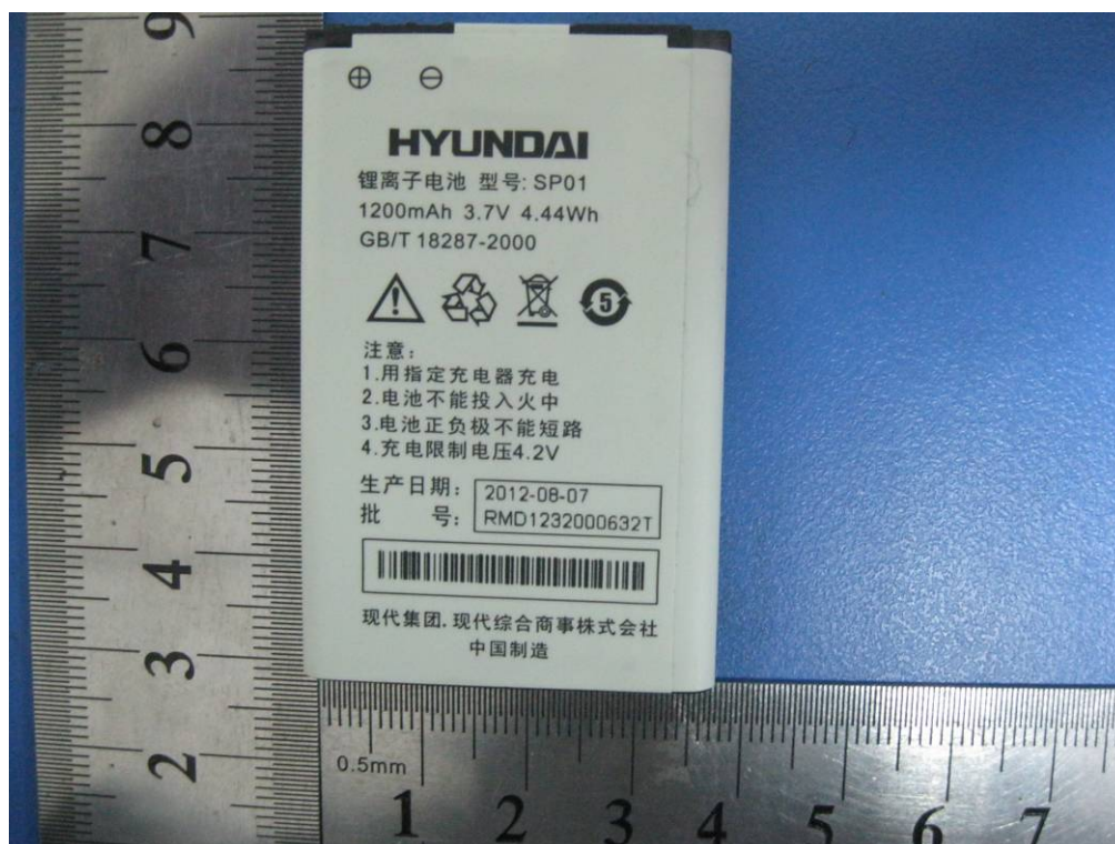
Battery - Top View
