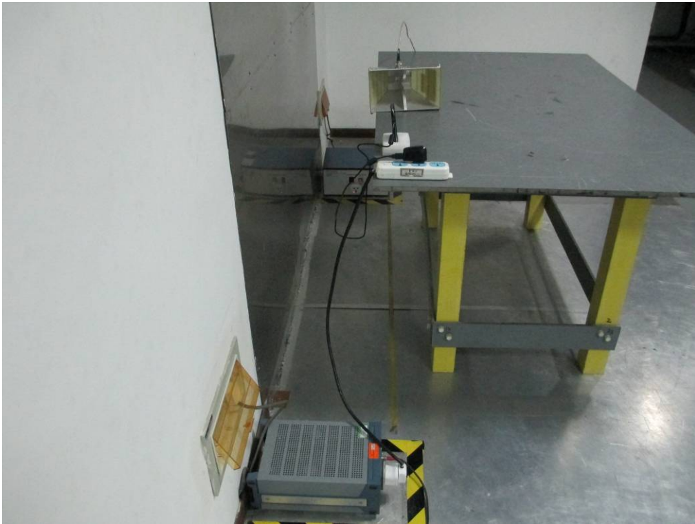
Conducted Emissions Test Setup Side View
