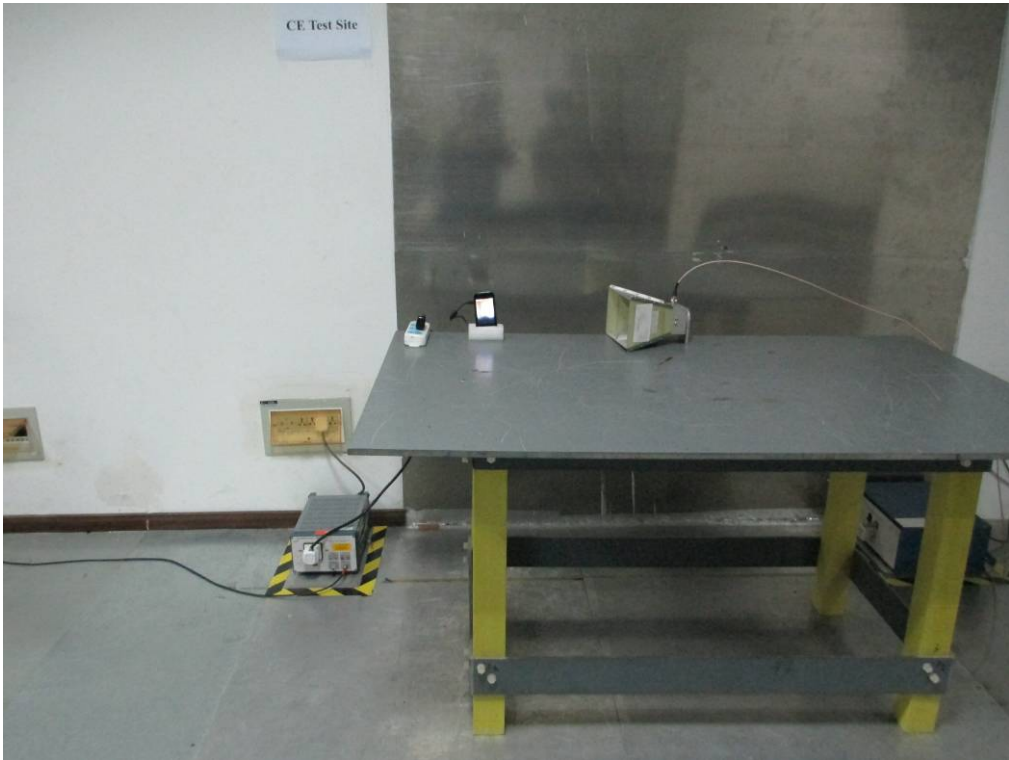
Conducted Emissions Test Setup Front View
