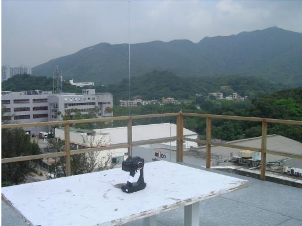
Measurement of Radiated Emission Test Set Up
