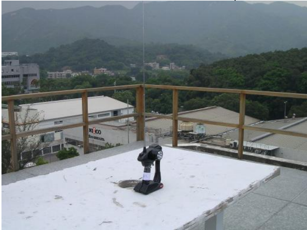
Measurement of Radiated Emission Test Set Up
