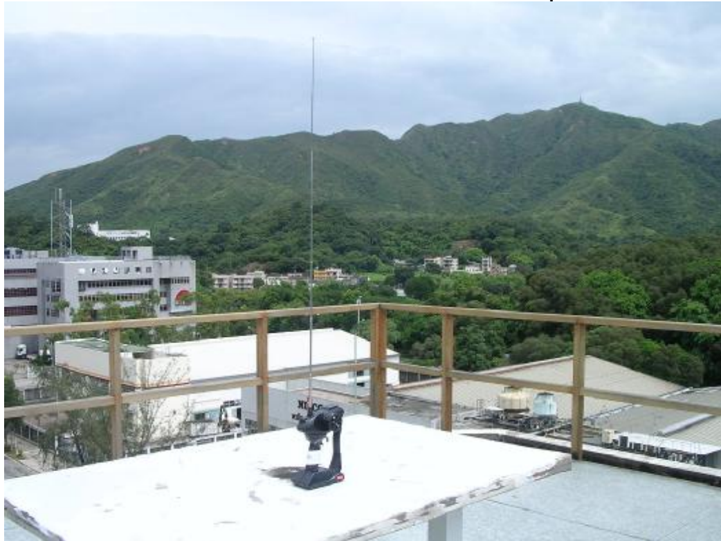
Measurement of Radiated Emission Test Set Up
