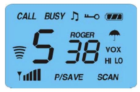
a. RSSI (Receiving Signal Strength Indicator) Icon Indicates the receiving signal strength
