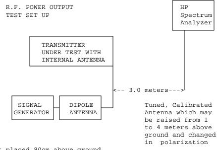
Equipment placed 80cm above ground on a rotatable platform.
